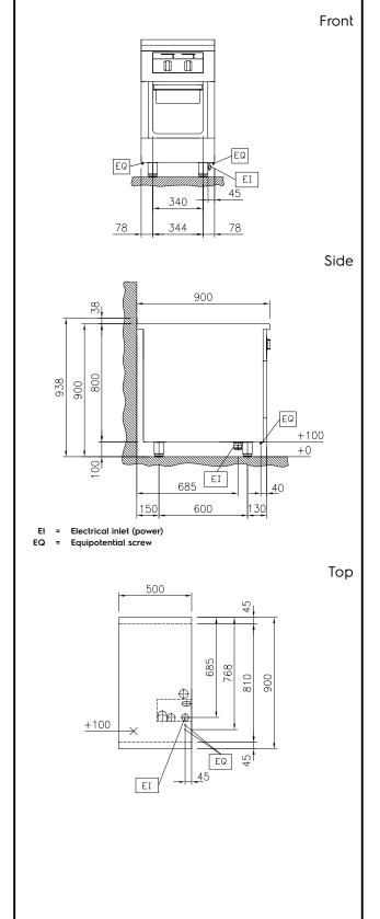
Electric Supply voltage: 400 V/3N ph/50/60 Hz Total Watts: 6 kW **Key Information:** 80 °C Working Temperature MIN: Working Temperature MAX: 350 °C External dimensions, Width: 500 mm External dimensions, Depth: 900 mm External dimensions, Height: 800 mm Net weight: 98 kg On Base;One-Side Operated Configuration:
